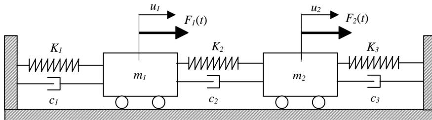
Figure 1 - Two-degree of freedom Duffing oscillator.
